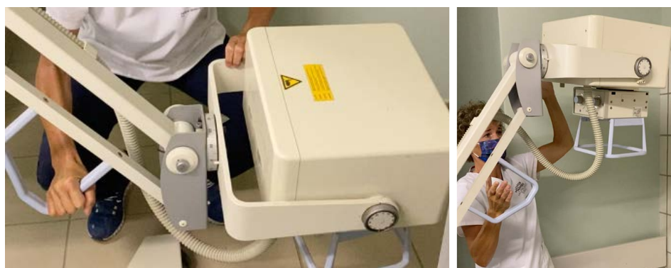
Fig. 12. The mechanism that should hold the extension column of the mobile X-ray unit in its proper position was again malfunctioning; the device could easily be stabilized manually (images from Mission 22-1 (March/April 2022).
