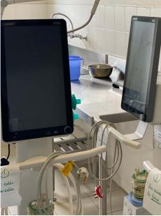
**Fig. 13.** ResVent<sup>®</sup> iHope at Rundu State Hospital: only 1 out of 4 machines passed both flow and oxygen calibration tests.
