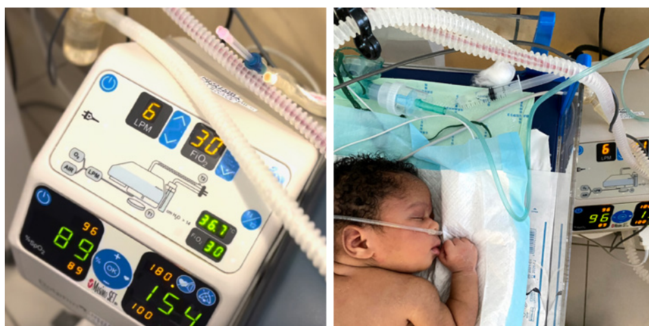
Fig. 5. MTTs Dolphin® CPAP machines with integrated Masimo® SET pulse oximeters: new patient cables allow the use with the new pulse oximetry sensors (RD SET NEOPT ADH SENS).
