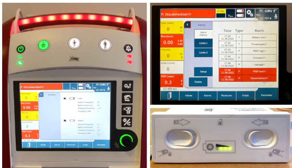
Fig. 4. Equipment maintenance: despite a fully charged external battery (right bottom), it was noted that the EVE® TR neo ventilator did not function properly because of internal battery malfunction.
