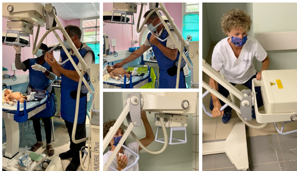
Fig. 22. The mechanism that should hold the extension column of the mobile X-ray unit in its proper position above the patient was malfunctioning; the device could easily be stabilized manually.
